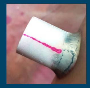
Fast and cost-efficient inspection of surface defects or porosity.
