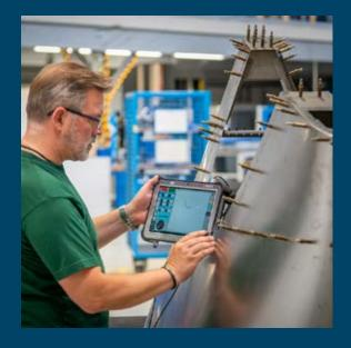
Surface inspection of delamination, thickness and conductivity.
